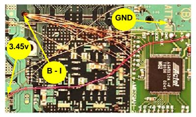
Note the position on the PS2 motherboard topside of the hole through which wires **BCDEFGHI** are to pass. (See picture to the left). Ensure you have enough wire length to run from the CD/DVD Controller vias on the underside, through the hole to the Messiah 2 chip (see photograph below). You are advised to solder to the vias first, and then pass the wires through the hole.
