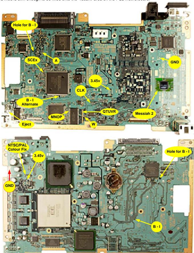
It is recommended that you solder to the PS2 motherboard first and then connect each wire to the appropriate point on the Messiah 2.
