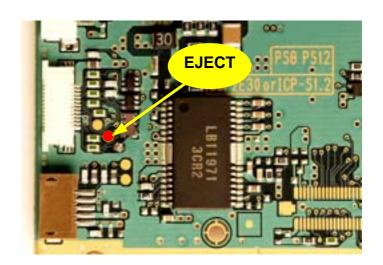
Now connect the  ${\bf A}$  wire as per the photograph to the left. (SCEx is shown for positional reference).
