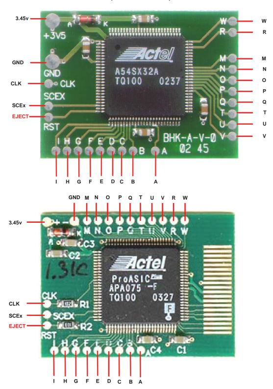
The **low resolution photographs** are for positional orientation (rather than magnification). The Messiah 2 mod is slim enough to be fixed onto the 'vacant' area on the PS2 motherboard.
