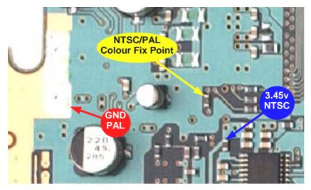
If you have an NTSC TV the Colour Fix point is taken to 3.45v. It forces NTSC colour on all PS2 game output. All PAL games will then be put out in NTSC colour mode and all PS1 games will display proper NTSC colour. The frame rate for PAL games will remain at 50 Hz.
