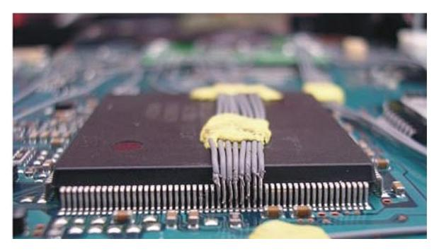
When this is done, **Messiah 2 wiring to the motherboard is complete** and the connexions can be made to the Messiah 2 with reference to the Messiah 2 Schematic.
