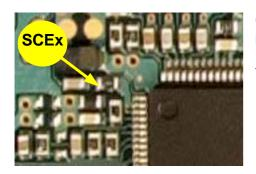
Care should be taken to ensure that the **SCEx** signal wire is properly soldered to its correct location on the resistor; the bond must be good (without damaging the resistor). This signal is used to boot PS1 backup games.
